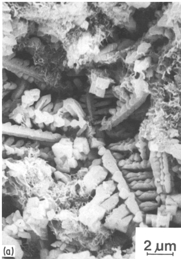
Figure 4 Appearance of heat-treated and then leached samples — scanning electron micrographs. (a) Pt/Rh crucible melt, sample 3; (b) Al 2 O 3 crucible melt, sample 4.
